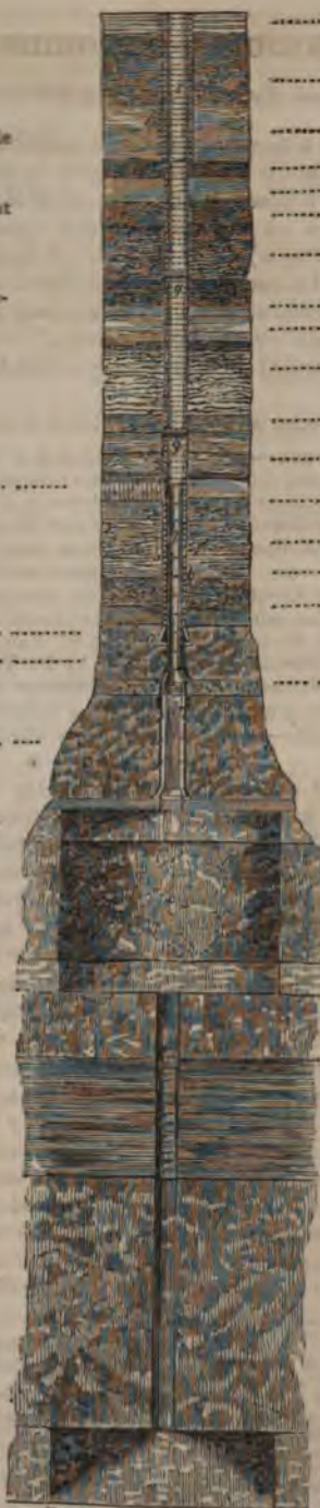
Section of the Wharfedale Salt Mine, on the River Weaver, Cheshire.
